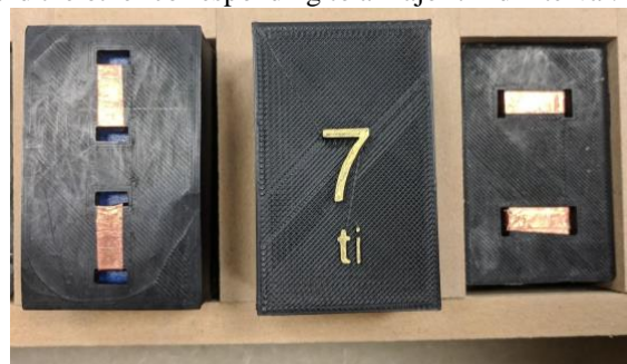
Figure 3: Resistor detection method for bass notes.
