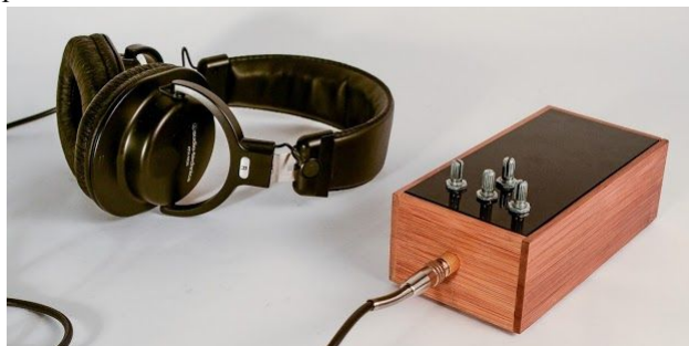
Figure 3: The noise machine has four potentiometers, without any instructions of how these modulate the sounds.
