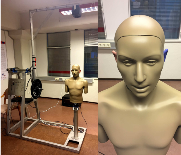
Figure 1. The used HRTF measurement system and room (left); detail of the KEMAR with custom left pinna (right).
