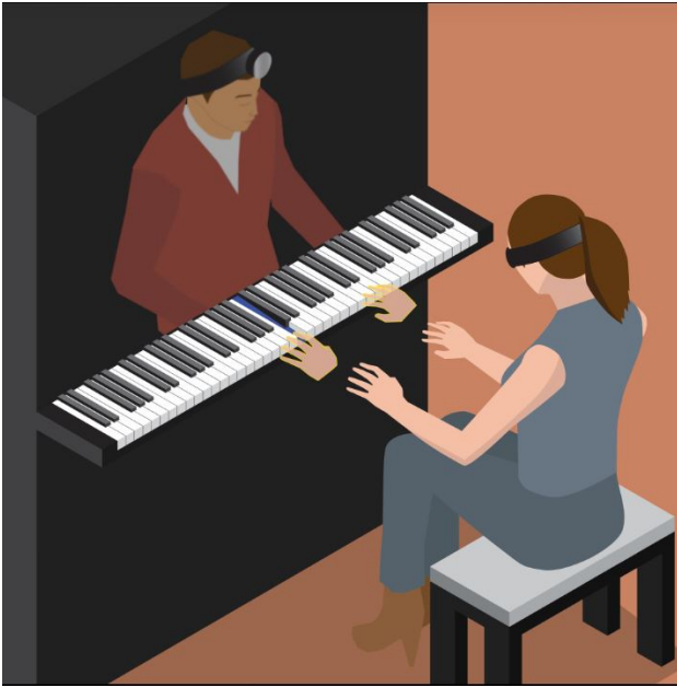
Figure 3. This figure is a model representing what the user sees inside the headset in the Mixed Reality environment. The user sees the virtual hands of the teacher on top of the physical keyboard. There is a blue highlight on the currently pressed key. The user also sees the face and upper body of the pianist in the reflection on the upright grand piano.
