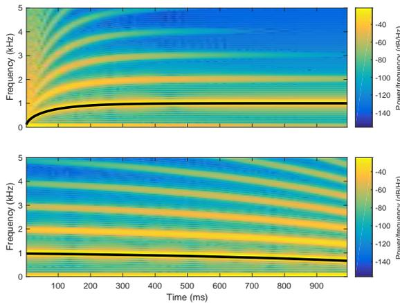
Figure 8. The spectrum of  $z_0(n)$  with time-varying argument  $\theta_0(n)$  overlaid with fundamental frequency  $f_c \sqrt{1 - B(n)}$  (dark curve) for  $B(n) = g^n$  (top) and  $B(n) = kn + l$  (bottom), validating use of  $\theta_0(n)$  in  $z_0(n)$  for known functions  $B(n)$  and showing sounding frequency of loopback FM can be accurately predicted.
