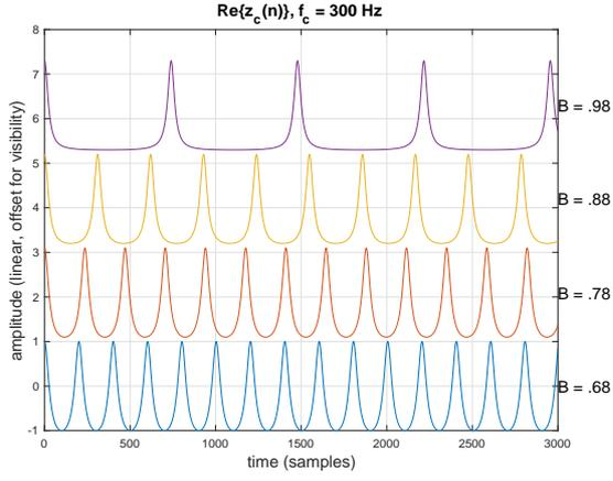
Figure 3. The real part of  $z_c(n)$  given in (50) is plotted (with offset) for 4 linearly spaced values of  $B$ , showing a *nonlinear* relationship to resulting period in samples  $M$  (and sounding frequency  $f_0 = f_s/M$  Hz,  $f_s = 44.1$  kHz).
