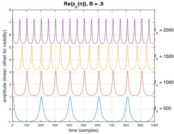
Figure 4. The real part of  $z_c(n)$  given in (50) is plotted with 4 linearly spaced values of  $f_c = \omega_c/(2\pi)$  showing a *linear* relationship with resulting period in samples  $M$  (and sounding frequency  $f_0 = f_s/M$  Hz,  $f_s = 44.1$  kHz).
