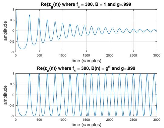
Figure 7. Waveform  $\Re\{z_g(n)\}$  (top) show that introducing a scalar multiple  $g$  to the loopback FM equation (69) introduces a change in both sounding frequency and amplitude. Waveform  $\Re\{z_c(n)\}$  (bottom) shows that setting the feedback coefficient to  $B(n) = g^n$  produces the same pitch change but without imposing an amplitude envelope.
