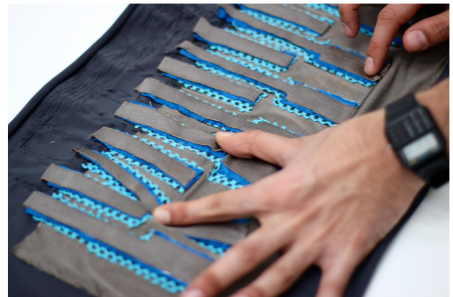
Figure 6. The fabric keyboard is built with multi-layer textile sensors machine-sewn in a keyboard pattern [35].
