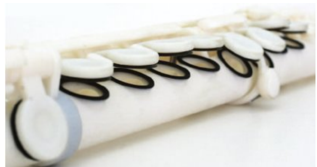
Figure 2. The 3D printed flute manufactured with the PolyJet technology [10].
