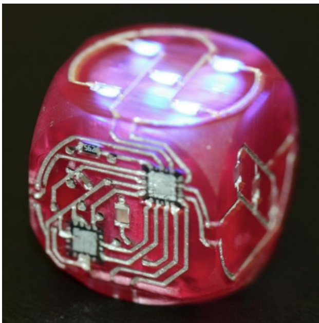
Figure 7. Gaming dice with electronic circuit mechanically designed into substrate. It consists of a micro-controller, MEMS accelerometer, batteries and LEDs [40].
